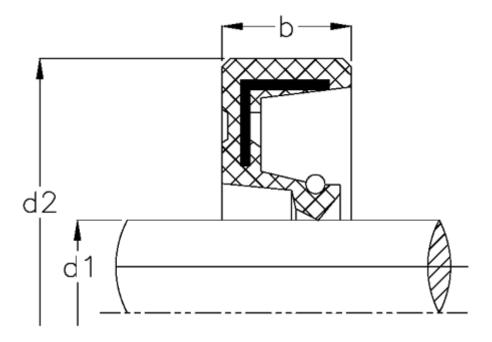
$\begin{array}{ll} b & = 7 \\ d1 & = 22 \\ d2 & = 32 \\ Material = NBR \end{array}$
